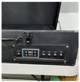
The box has a lid made of 1"x3" stock and 1/4" plywood. Both the base and the lid sides are mitered 45°
